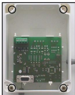
Picture 5 - wall fixing screw holes
